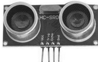
Gambar 2.3 Sensor Ultrasonik HC-SR04 Sumber (Wicaksono MF: 2017)
