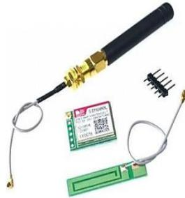
Gambar 4. Modul SIM800L Quad Bank GPRS GSM
