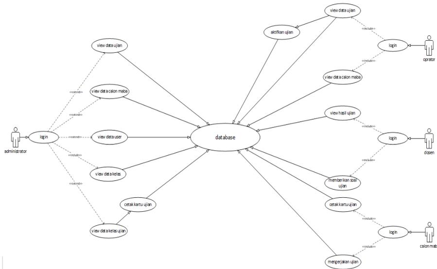
Gambar 1. Diagram Use Case Sistem Computer Based Testing
